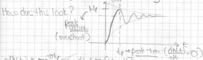
$$\frac{dh(t)}{dt} = \cancel{\sigma e^{-\sigma t} [\cos \omega_d t + \frac{\sigma}{\omega_d} \sin \omega_d t]} - e^{-\sigma t} [-\omega_d \sin \omega_d t + \sigma \cos \omega_d t]$$
