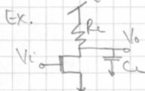
$$A_v = -g_m Z_{out} = -g_m \left( \frac{R_L}{1+sR_L C_L} \right)$$
