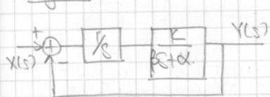
$$H(s) = \frac{Y(s)}{X(s)} = \frac{\text{feed forward gain}}{1 + \text{loop gain}}$$
